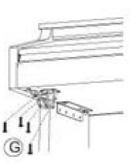
Headphone Holder Installation: Attach the headphone holder to the bottom left of the piano with the four Headphone Bolts(G).
